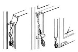
Pull the mechanism down about 150mm without allowing it to untwist and lose the spring's tension. Turn the tool two or three times anti-clockwise to add tension, then hook it back in place.
